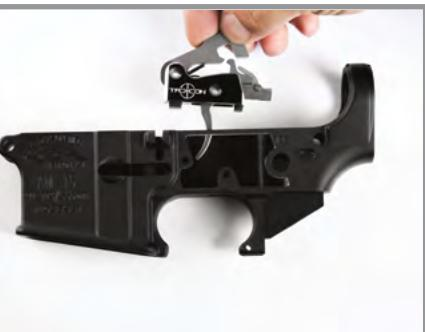
Prior to installing the 3MR, ensure all previous trigger components and selector have been removed. To remove the selector, uninstall the grip and remove the selector spring and detent. Use care to ensure you retain these parts. The 3MR will "drop in" as shown.
