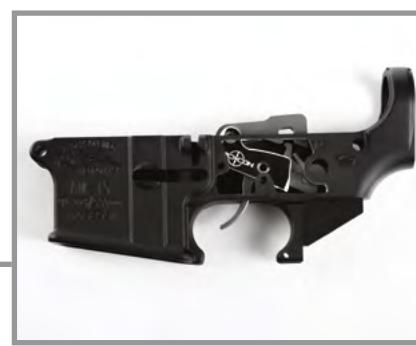
Allow the 3MR to drop in completely, making firm contact with the bottom of the receiver. Verify proper fitment by visually confirming the hammer and trigger pin holes align properly.
