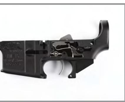
If you ordered an ambidextrous selector, choose your preferred paddle sizes and configuration. Fasten one paddle then install the selector assembly into the receiver. If you ordered a standard selector, verify the paddle is secure and install. When installing the selector, rotate the fore end of the trigger pack up to allow clearance.
